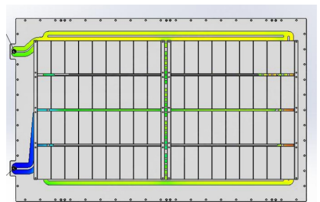
Battery pack bottom plate liquid cooling simulation
